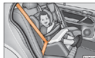
Fig. 146 Child seat with padded table in Group 1 installed on rear seat bench facing the direction of travel
