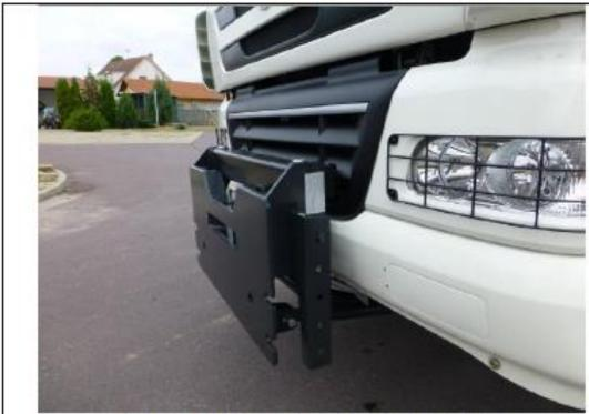
Figure 5 - front fixing plate, protection of the running light
