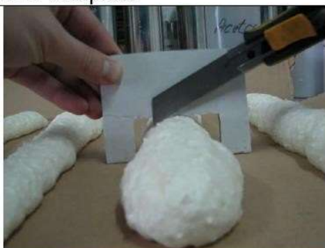
Figure 3: How to find 3 cm diameter bead
